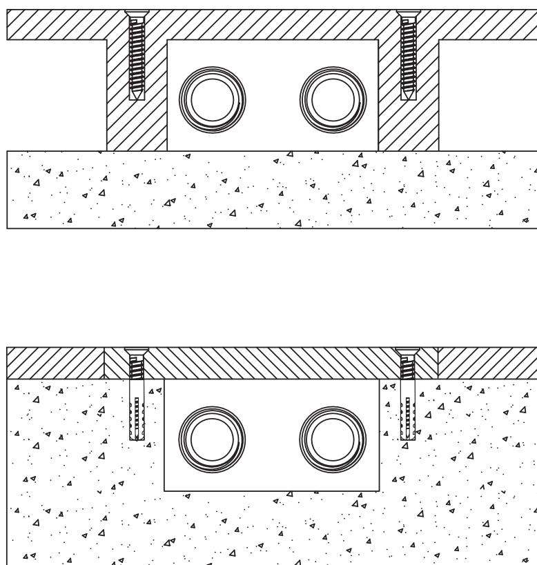
**EN** Representative drawing of the space allowing the passage of hoses.
