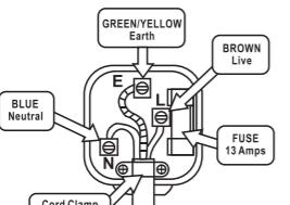
As the colours of the wires in the mains lead of this appliance may not correspond with the coloured markings identifying the terminals in your plug, proceed as follows.
