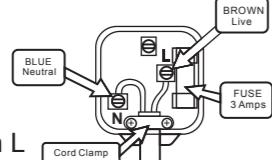
WARNING: Never connect live or neutral wires to the earth terminal of the plug.
