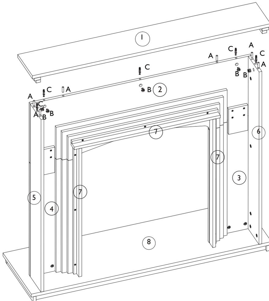
Insert 5x cam locks (C) and glue (J) 6x wood dowels (A) into the legs, side panels and front panel (2,5,6)
