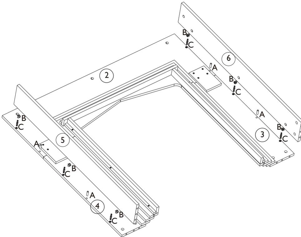
Use the glue (J) in the dowel holes before inserting 2x dowels (A) into the left and right hand panels (3)(4). Position the cam bolts (C) in to left and right side panels (3)(4).
