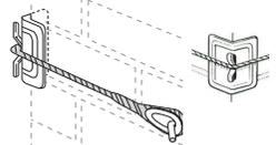
Fix the remaining cable eye over the other J bolt. Then fold the loose end of the lashing cable around cable eye and fix as described in instruction above. Tighten both J bolts and nuts to secure the chimney fixing bracket.
