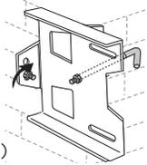
Fold one end of lashing cable (C.) around one cable eye (D.) leaving a 100mm surplus end. To fix lashing cable to cable eye, separate the individual wires in the cable's surplus end and wrap them one at a time, around the main cable. Then hook the cable eye over the J bolt.
