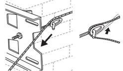
Lastly, fix the aerial mast to chimney fixing bracket using V bolts and nuts (F). Tighten firmly to secure.
