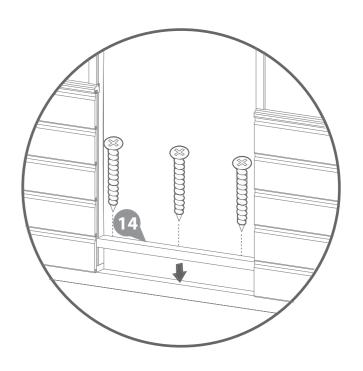
Fix the Gable tops (No. 4)& (No. 5) to the panels using 4x50mm screws per top as shown in the diagram.
