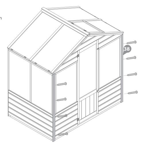
Fit the fascias (**No. 10**) and the finials (**No. 21**) to the building using 14x30mm screws as shown in the diagram.
