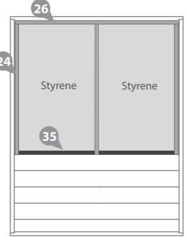
Fix the corners of the Sml Window Side (No. 2) and the Lrg Window Side (No. 3) with 3x50mm screws as shown in the diagram.
