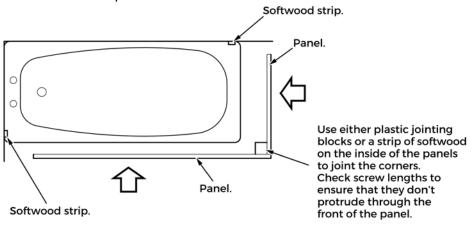
Note: Plastic jointing blocks, corner posts, softwood strips and screws are not supplied.
