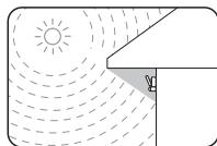
**EN** Avoid sunlight falling onto the lens of sensor
