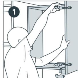
1 To decide the height, make sure you're clear on how you'll position the cornice pelmet and how it joins to your end panel. Clamp panel into place with 2 cm overhang at the front edge.
