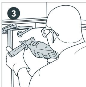
3 Drill through from the back with a piece of timber clamped to the front of the door. This prevents the drill bit from damaging the finish.
