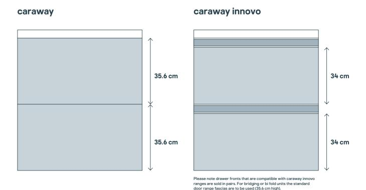
While the standard caraway kitchen cabinets are compatible with many drawer configurations, the caraway innovo handleless system is designed with more aesthetically pleasing lines so only highline and 2 drawer options are available. However, that does not stop multiple drawer combinations being achieved with the 2 drawer fascias being able to create 2 drawer, 3 drawer and 4 drawer configurations using internal drawers with the 2 drawer fascias.
