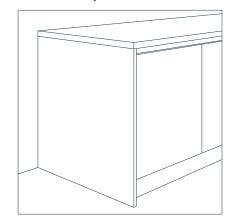
Floating end panels are created using an external corner post, outer worktop corner joint, clad on / tall housing spacers, floating clad on rail to cabinet fixing bracket, worktop rail and external floating end panel. When creating a peninsula unit / island a second external corner post and outer worktop corner joint are required.
