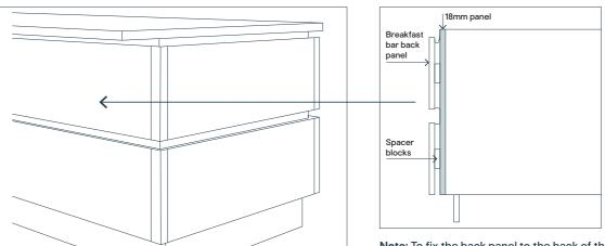
**Note:** To fix the back panel to the back of the Innovo cabinets when using a rail an 18mm panel will need to be attached to allow the spacer blocks to be fixed and the back panel fixed to them.
