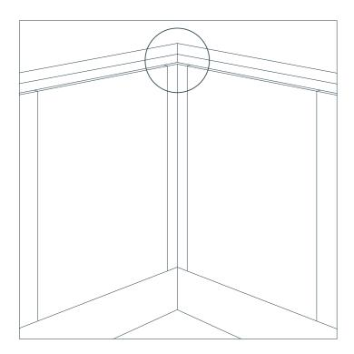
$\textbf{1.} \ \ \textbf{Take your rail and cut it to length, using the internal corner joint to join.}$
