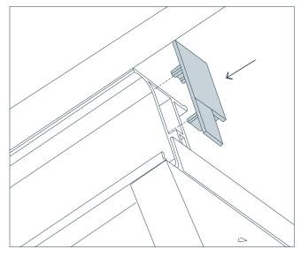
Vertical end caps can be easily adapted to fit both vertical end and vertical middle rail options. Simply snap to adapt.
