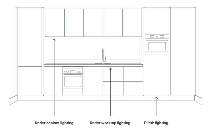
The standard under cabinet lighting is not compatible with the caraway innovo handleless kitchen cabinets. Instead please use the specially created dotless LED warm white striplight kit (5m).
