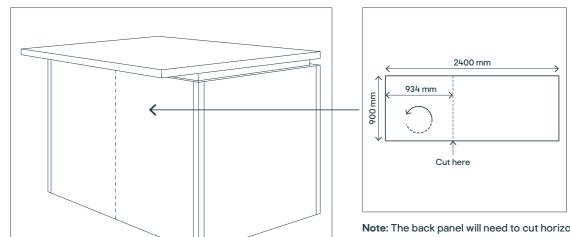
Note: The back panel will need to cut horizontally at 934mm, turned round and joined to become the correct height if a rail and plinth are not used with Innovo cabinets.
