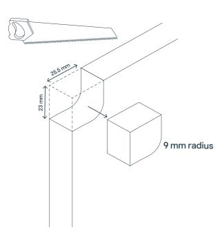
Note: The base of the cabinet will need to be removed, cut and then used to strengthen the now top of the cabinet. Notches will need to be cut to accommodate the worktop rail. Additional feet and raisers will also need to be purchased. Please refer to the instruction manual for full details.
