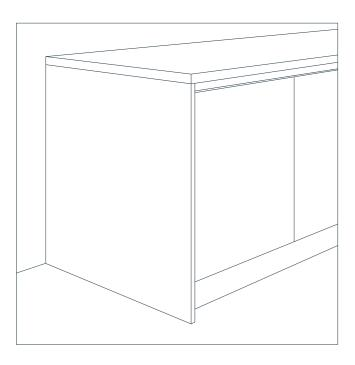
Fitting a clad on end panel on a caraway innovo handleless cabinet is exactly the same as on a standard caraway cabinet. The main steps are about measuring where you need to cut your panel at the rear of the unit and along the top. Please refer to the step by step instruction manual.
