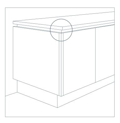
1. Carefully measure and cut the return section of the worktop rail. Remember to allow an additional 4 mm for the corner joint itself.
