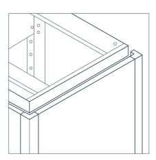
2. Take the rail for the return section and fit the corner piece to it. Then position it on the side of the cabinet whilst connecting the corner piece into the front rail.
