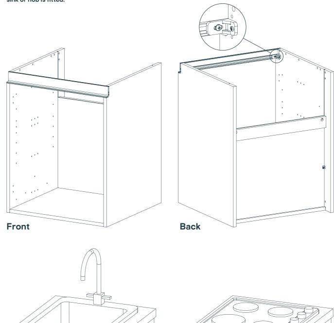
**Note:** The front top brace will need to be removed and the rear support bar located in the middle of the cabinet. Additional right angle fixing brackets will also need to be purchased. Please refer to the instruction manual for full details.
