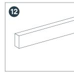
This 25 mm thick batten is used behind base, tall larder, appliance housings to ensure the cabinets are spaced enough away from the wall.
