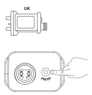
**EN** To set and reset the timer, press button: 6 hours on / 18 hours off. Green light on = Timer is on
