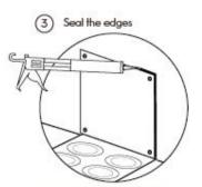
Use the Clear Silicone Sealant to seal around all four sides of the splashback. Take care to ensure that the sealant is no more than 2.5mm in thickness.
