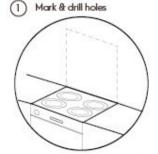
Decide Where you Want to position your splashback, then carefully and accurately mark where the drill holes need to be. Select the correct sized drill bit and determine depth of hole required. Once drilling complete, insert Wall plugs firmly into holes.
