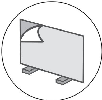
Make sure all corners are well protected from any hard surfaces. Carefully peel off the protective film back. Take care not to remove the self-adhesive backing.
