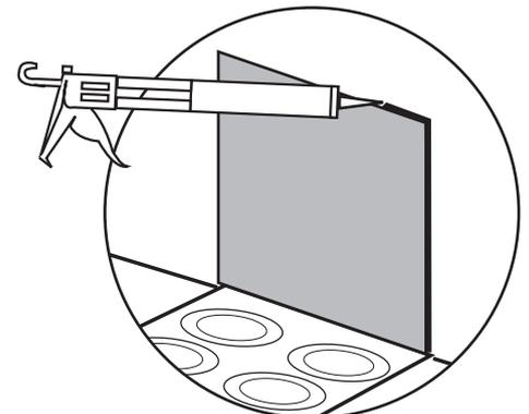
Use the Clear Silicone Sealant to seal around all four sides of the splashback. Take care to ensure that the sealant is no more than 2.5mm in thickness.
