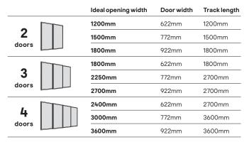
Top track H39 x D91mm. Bottom track H7 x D65mm
