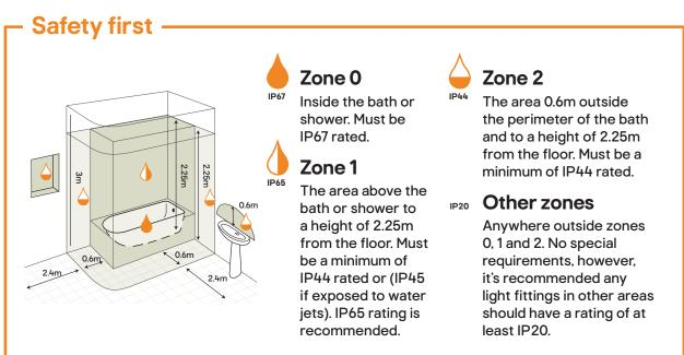
A 30mA RCD must be used. All new and modified electrical installations must comply with the latest IET Wiring Regulations (BS7671) and bathroom lighting products must be installed in accordance with local Building Regulations. If you are in any doubt, contact a qualified electrician.
