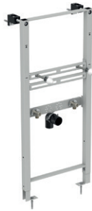
Ideal Standard ProSys frame for wall-hung basins with deck-mounted taps W500 x H1150 x D40mm For built-in or plasterboard wall installation. Pre-assembled frame for wall-hung wash basin. Easy and quick installation. Height adjustable 0mm-200mm. 3391500579613 €259
