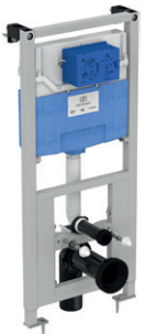
Ideal Standard ProSys pneumatic flush cistern and adjustable 3-height wall-hung toilet frame W500 x H1150 x D150-210mm Pneumatic actuation. Water-saving smart valve (delay fill). Easy adjustment to low water volume. 5017830550013 €412
