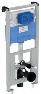
Ideal Standard ProSys pneumatic flush cistern and adjustable 3-height wall-hung toilet frame W500 x H1150 x D150-210mm Pneumatic actuation. Water-saving smart valve (delay fill). Easy adjustment to low water volume. 5017830550013 €412
