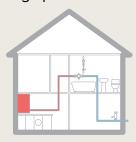
You have a boiler unit but no hot water cylinder, the boiler unit is usually found in the kitchen and delivers hot water on demand.
