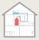
You have a cold water tank in your attic and a hot water tank in your airing cupboard. You can choose any of our low pressure taps (minimum operating pressure of 0.1 – 0.5bar).
