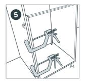
With the larder cabinet in position, adjust the height, so that the bottom of the larder cabinet is level with the bottom of the standard base cabinets.
