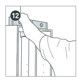
For blind corners, hang the wall cabinet onto the brackets, and level to the top line by using the cabinet adjusters inside the cabinet. Fit the adjacent cabinet and allow for the 5.9 cm corner post. Secure the corner post to both cabinets using connecting blocks.
