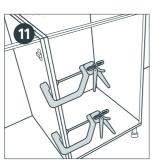
Use quick release clamps to clamp the cabinets together. Mark holes through the wall brackets at the back of each cabinet, drill holes and insert suitable wall plugs.
