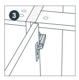
Use the adjustment screws to align the doors perfectly with the cabinets and other adjacent doors. Alignment can be in numerous directions.
