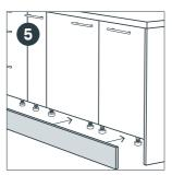
A plinth offers a finish to the bottom of kitchen cabinets and covers the gap between the floor and the bottom of the base cabinets.
