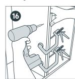
Drill through cabinets and use cabinet connectors to secure them together. Hide screws behind hinge plates.
