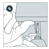
Repeat the cutting and assembling of the mitre joints for the pelmet and secure with screws by screwing through the back lip up into the bottom of the wall cabinets.
