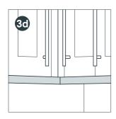
A light pelmet can be used in a corner by cutting a 45 degree angle as pictured above.
