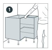
Start by fitting the corner base cabinet by aligning it with the wall markings.
