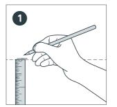
Measure up 53 cm from the top of the base cabinets and put a mark on the wall where the wall cabinets are going.
