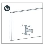
Using the screws provided, fit the connecting brackets to the drawer fronts, onto the pre-marked fixing positions (the pre-marked holes will vary depending on the type of drawer front - deep pan, standard etc).
