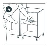
For blind corner cabinets only: Connect the two cabinets together using a 5.9 x 5.9 cm corner post, attaching the post with connecting blocks.
