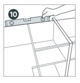
Level each cabinet as you go, ensuring they align with the 87 cm line on the wall.
