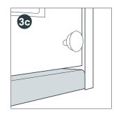
A light pelmet can run into an end panel at the end of a cabinet run. You will need to cut the end panel so it carries on past the bottom of the door.
