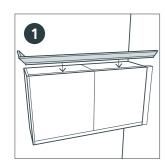
A cornice offers a finish around the top of your wall cabinets. Cut the cornice to fit using a mitre saw to create the internal and external mitres.
