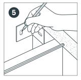
Mark the wall through the wall fixing brackets attached to the cabinet.
