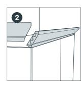
Cut the mitre on each cornice using a mitre block and saw. Use mitre adhesive to secure mitre joints together. Secure the cornice to the cabinets by adding screws through the back lip of the cornice and into the top of the wall cabinet.
