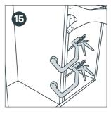
Use quick release clamps to clamp the cabinets together, ensuring their front edges are level with one another. Once the run of cabinets is straight and level. tighten the bracket adjusters from the inside to ensure they do not move
