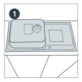
Cut the sink and hob holes in the worktop. This is done by positioning the worktops in place and laying the sink and hob in position to ensure that it
