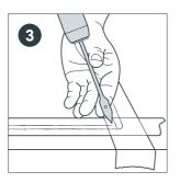
Remove the worktops, place on trestles and cut out the holes by drilling into the corners where the lines meet. Use a large enough drill bit to give access for a jigsaw blade.
