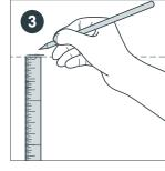
For standard wall cabinets, measure up 72 cm from this line and mark the wall again. Use a spirit level on the 72 cm mark and draw a horizontal line across the wall (this line simulates the top of the wall cabinets and will be at 90 cm for tall wall cabinets).
