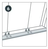
Cut the plinth to length and attach the leg clip plates to the back of the plinth in line with the cabinet legs. Attach the leg clips to the plates and then place the plinth in position and push until the clips locate over the kitchen cabinet legs.
