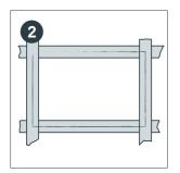
Apply masking tape to the outside area where the hob and sink are positioned. Then use the provided template or measurements to mark on to the masking tape.
