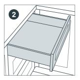
Position drawer boxes onto their runners and ensure they open and close smoothly. Drawer fronts will be fitted later when the kitchen doors are fitted.
