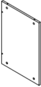
(B) -1: Middle Side-board (x2) 565*400*15mm
