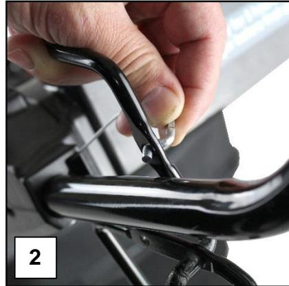
3.15 Follow the curve of the cable until the cable lies flat in the handle (1).
