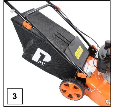
2.9 Gently pull the recoil start handle (1) up to the recoil retaining loop (2).
