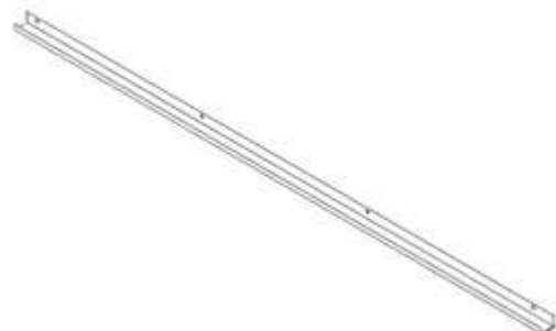
G04 GUTTER - A4M01999 (x2) 1 9/16"x1 15/16"x79 7/16" (40x50x2017)
