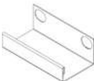
G05 GUTTER SPLICE - A4M02004 (x2) 1 7/16"x2 1/16"x3 15/16" (36x52.5x100)
