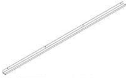
G03 GUTTER - A4M01998 (x1) 1 9/16"x1 15/16"x79 7/16" (40x50x2017)
