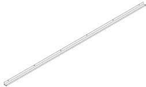
G01 GUTTER - A4M01993 (x2) 1 9/16"x1 15/16"x108 7/8" (40x50x2765)
