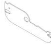
L03 LOUVER SIDE PLATE - A4M04138 (x46) 1/16"x2 3/16"x6 9/16" (2x55x167)
