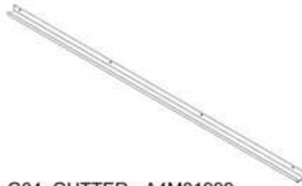
G04 GUTTER - A4M01999 (x1) 1 9/16"x1 15/16"x79 7/16" (40x50x2017)
