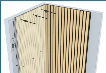
Method A: Using an appropriate anchor system for the wall, screw the acoustic panel in place. Leave a 600mm gap between each row. Sound absorption class: D
