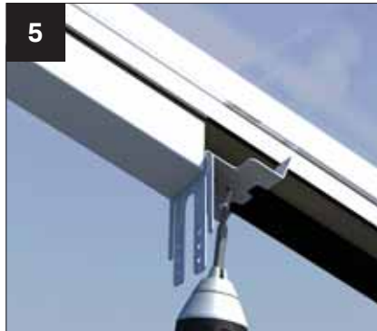
5 Take the transom bracket (CHA001) and attach using two 4.2 X19mm self-drill pan head screws (supplied). The back edge of the bracket should butt up to the under cladding.
