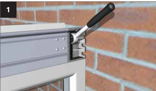
1 Where the eaves beam sits against the host masonry wall, it has a structural moulding attached to the eaves beam. This has three fixing positions cast into it to allow attachment into masonry – choose the hole that directly lines up with solid masonry and drill a 10mm hole into the host wall. Attach the structural moulding using the M8x80mm anchor supplied. Silicone seal the gap where the moulding attaches to the eaves beam.
