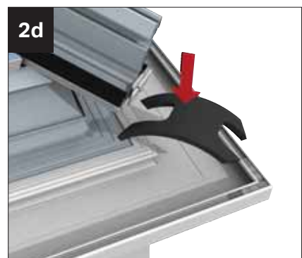
2d At 90° corner insert 'H' section and press down. Similarly apply at stop end or outlet positions.
