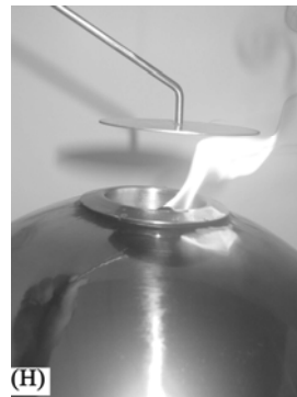
H). Quench-fire cover (h) is used for extinguishing flame, cover it on flame, it goes out.
