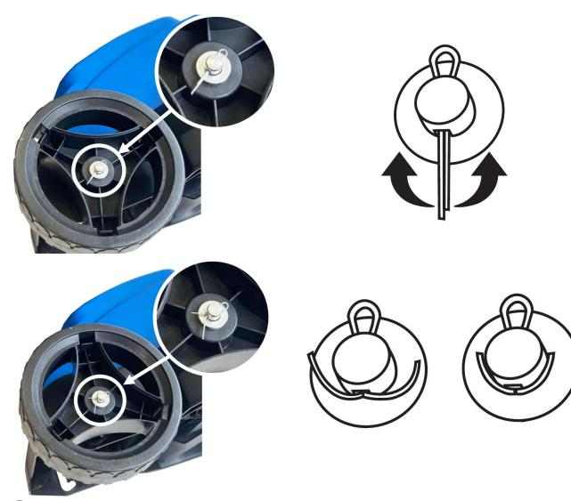
4 Fit a wheel cover onto the wheel and clip into place.
