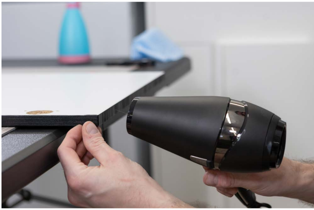
Use a hairdryer to help secure the film around the corners and edges
