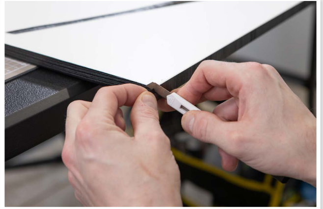
Fold the second flap around the corner and trim away excess film
