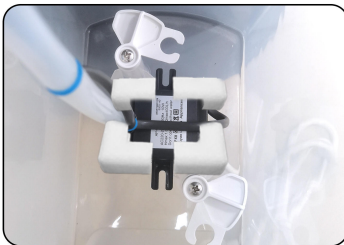
1. Remove the foam around the pump
