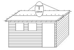
Roll the felt onto the roof, if you have more than one length of felt begin at the lower part of the roof. Make sure that felt is overhanging three sides of the shed. Start at one end, using the 10mm clout nails, fold the felt over the side of the roof and secure with clout nails. Work your way along the roof, taking care to remove wrinkles in the felt as you go. Use one clout nail every approx. 20cms.
