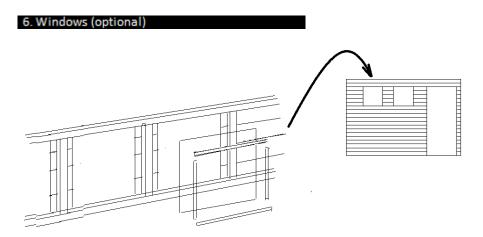
To fit the windows it is recommended that a waterproof sealant is applied around the edge of the glazing before fitting. From the inside of the building fit the styrene window into the frame and secure in place with the 4 strips of window bead. Fix the window bead to the window frame with 30mm panel pins.
