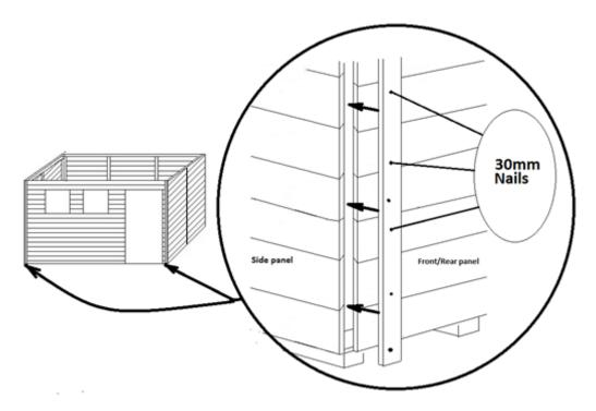
Position the corner cover strips as shown above and fix with 30mm nails.
