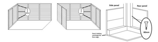
Secure the rear and side panels together as shown above, using 60mm screws. Note that the framework of the panels rests on the floor with the cladding over hanging. Continue until all sides including the front panel are in place and fixed together.
