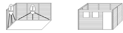
When all sides of the shed are upright and screwed together, use the 60mm screws to secure the side to the floor as shown above.
