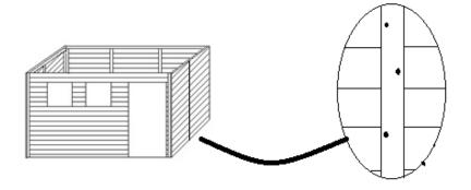
Position the joining strips over the side joins in the shed panels and fix with the 30mm nails as shown.
