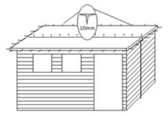
Roll the felt onto the roof, if you have more than one length of felt begin at the lower part of the roof. Make sure that felt is overhanging three sides of the shed. Start at one end, using the 10mm clout nails, fold the felt over the side of the roof and secure with clout nails. Work your way along the roof, taking care to remove wrinkles in the felt as you go. Use one clout nail every approx. 20cms.
