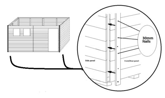
Position the corner cover strips as shown above and fix with 30mm nails.
