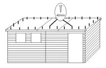
Align the roof so that it overhang s on all sides. Using the 40mm screws, fix the roof panel by screwing through it and into the framwork of the shed.
