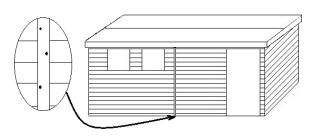
Place the joining strips over the front and rear joins in the shed panelsas shown and fix into place with the 30mm nails.
