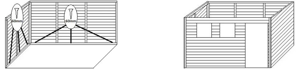
When all sides of the shed are upright and screwed together, use the 60mm screws to secure the side to the floor as shown above.
