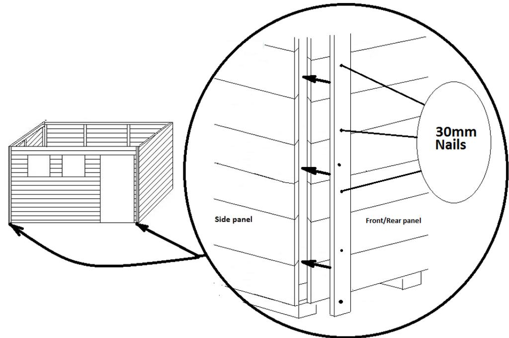
Position the corner cover strips as shown above and fix with 30mm nails.
