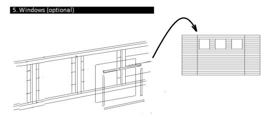
To fit the windows it is recommended that a waterproof sealant is applied around the edge of the glazing before fitting. From the inside of the building fit the styrene window into the frame and secure in place with the 4 strips of window bead. Fix the window bead to the window frame with 30mm panel pins.
