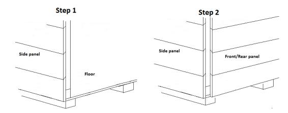
**Step 1**. Position the first side panel so that the edge of the panel is flush with the edge of the floor and the overhang on the bottom of the panel is butted up to the floor.
