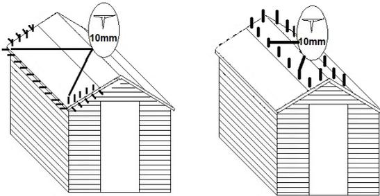
If the shed has more than two lengths of felt, position the first length along the lower edge on one side of the roof and fix as shown. Repeat on the other side of the shed. Place the final piece of the felt over the apex of the roof, ensuring that it overlaps the existing felt and fix with clout nails.
