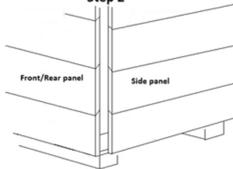
**Step 1.** Position the first side panel so that the edge of the panel is flush with the edge of the floor and the overhang on the bottom of the panel is butted up to the floor.
