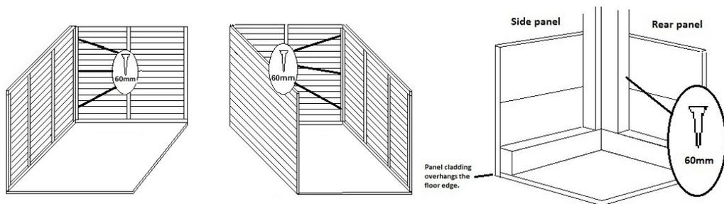
Secure the rear and side panels together as shown above, using 60mm screws. Note that the framework of the panels rests on the floor with the cladding over hanging. Continue until all sides including the front panel are in place and fixed together.
