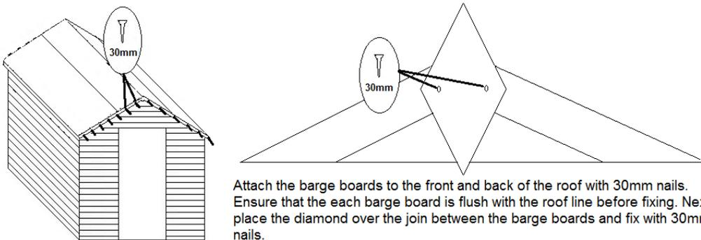
Attach the barge boards to the front and back of the roof with 30mm nails. Ensure that the each barge board is flush with the roof line before fixing. Next place the diamond over the join between the barge boards and fix with 30mm nails.
