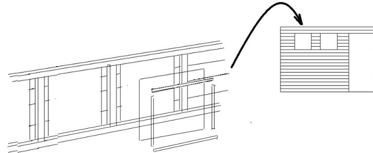
To fit the windows it is recommended that a waterproof sealant is applied around the edge of the glazing before fitting. From the inside of the building fit the styrene window into the frame and secure in place with the 4 strips of window bead. Fix the window bead to the window frame with 30mm panel pins.
