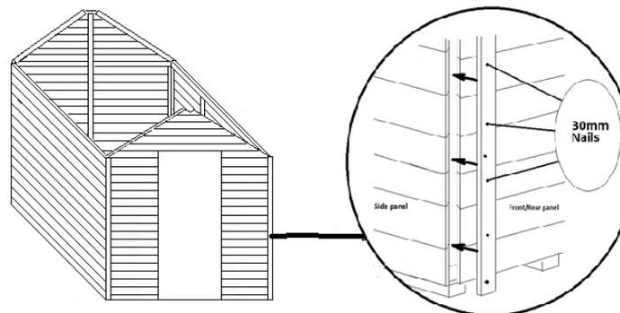
Fix the corner strips using the 30mm nails as shown above.
