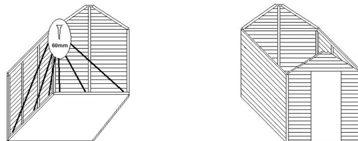
When all sides of the shed are upright and screwed together, use the 60mm screws to secure the side to the floor as shown above.
