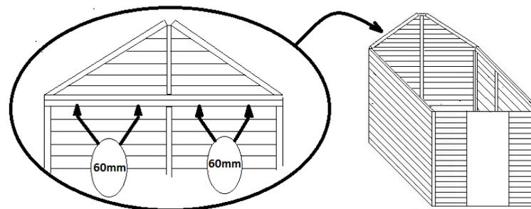
Position the front and rear apex panels on to the top of the front and rear panels. Fix the apex panels in place using the 60mm screws as shown above.
