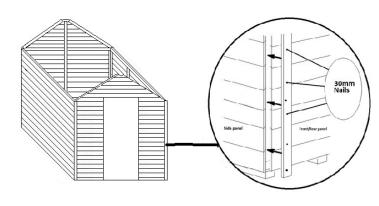
Fix the corner strips using the 30mm nails as shown above.
