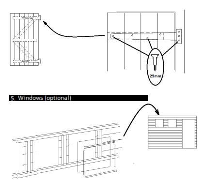
To fit the windows it is recommended that a waterproof sealant is applied around the edge of the glazing before fitting. From the inside of the building fit the styrene window into the frame and secure in place with the 4 strips of window bead. Fix the window bead to the window frame with 30mm panel pins.
