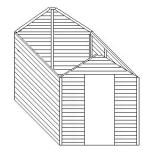
When all sides of the shed are upright and screwed together, use the 60mm screws to secure the side to the floor as shown above.
