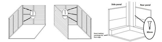
Secure the rear and side panels together as shown above, using 60mm screws. Note that the framework of the panels rests on the floor with the cladding over hanging. Continue until all sides including the front panel are in place and fixed together.
