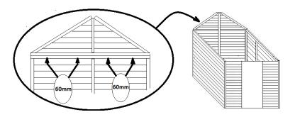
Position the front and rear apex panels on to the top of the front and rear panels. Fix the apex panels in place using the 60mm screws as shown above.
