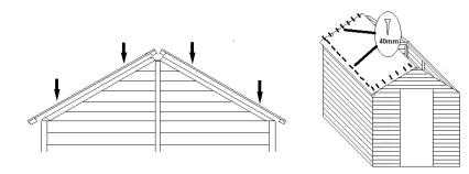
Lay the roof board on the shed as shown. Using the 40mm screws, fix the roof into position by screwing through the roof panel into the framework of the shed.
