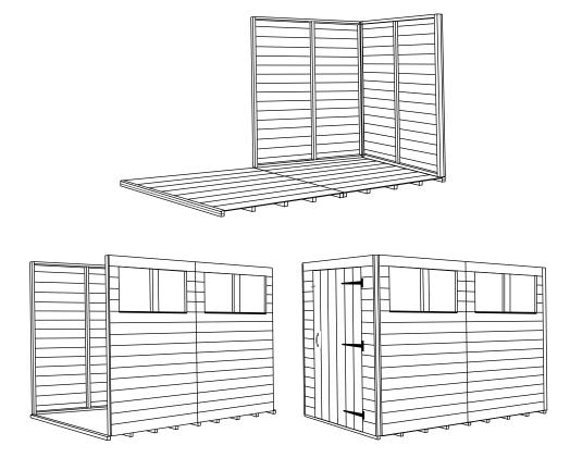
**d.** Once all of the side panels are fixed together you can then attach the sides to the floor by screwing through the bottom internal frame into the floor panel, using 60mm screws.
