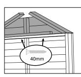
**b.** Attach the gable tops to the gable end panels (the panels which are on the heavy-duty bearers) by screwing up through the internal framing using 40mm screws. Make sure that they are flush with the front and back of the panel.
