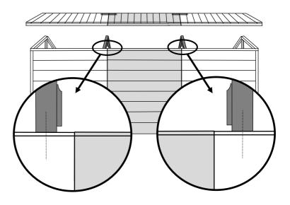
For sheds with more than 2 roof panels in length, position the apex supports so that the roof panels sit halfway across each support, fix with 50mm screws. Ensure that the finished roof will overhang the gable ends equally.
