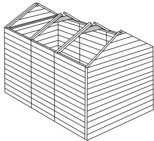
For sheds with multiple roof boards, attach the roof connector batons to the underside of the roof panels as shown using 50mm screws. For larger roofs 10ft and above the batons will need to be attached to both ends.
