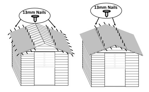
**a.** Starting with the lower part of the roof, attach the felt using the 13mm clout nails ensuring that there is a 30mm overhang around the edge. Next roll out and attach the centre piece of felt as shown above
