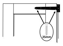
c. Attach the bolts to the top and bottom of the inside of the door which has no weather strip attached.
