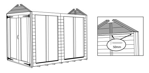
**b.** Attach the gable tops to the gable end panels (the panels which are on the heavy-duty bearers) by screwing up through the internal framing using 50mm screws. Make sure that they are flush with the front and back of the panel.
