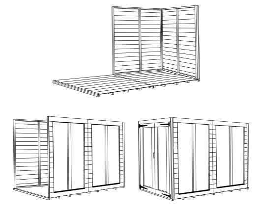
**d.** Once all of the side panels are fixed together you can then attach the sides to the floor by screwing through the bottom internal frame into the floor panel, using 70mm screws.
