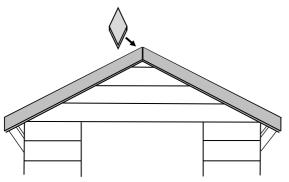
**b.** Attach the roof trim to the front and rear of the sheds using the 40mm nails.
