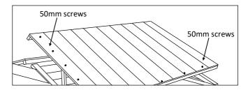
Once all of the roof boards have been placed onto the shed, screw the centre of the underside of the roof together.
