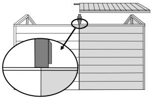
Lay the roof boards on top of the shed as shown, ensuring that the panels sit halfway across the apex roof supports, so that the next panel has space to fit onto the same support.
