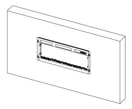
• Install the front glass panel back . Make sure the hook is fully hooked into the lock. The installation is completed now.
