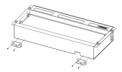
Hang the firebox on the wall bracket and mark the position of the L bracket ,then take the firebox down. Drill 2 holes on the marked point, insert 2 wall plugs into the holes, then hang on the firebox again and fix it by two ST5\*40 screws.
