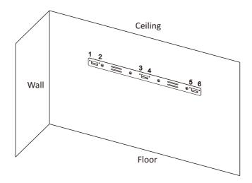
• Insert wall plug(for concrete wall only) into the holes and secure the bracket to the wall with six ST5\*40 screws.
