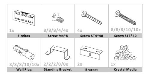
**Note:** Standing brackets are only prepared for EF449A/EF450A/EF451A.
