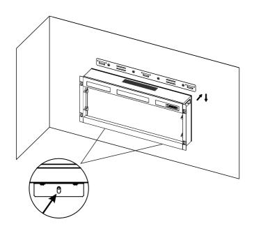
Repeat the steps mentioned above to arrange the fuel bed and install the front glass panel and fix it to the sides of firebox with the screws.
