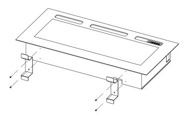
Repeat the steps mentioned above to arrange the fuel bed and install the front glass panel and fix it to the sides of firebox with the screws.
