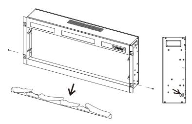
Insert the firebox into the framework and fix it by four ST4x40 screws
