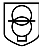
Safety isolating. Products with this symbol are designed so the output is electrically isolated from the unit.
