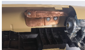
Position for storing thermal conductive plates
