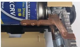
Connect the inner bracket to the tank surface
