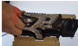
2.1 Lift the burner up
