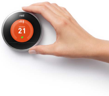
The Nest learning thermostat learns the customer's schedule to programme itself and automatically turns down the heat when they are out
